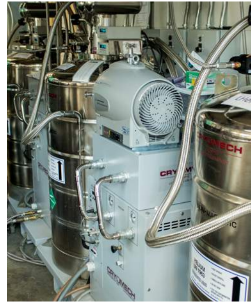
Laboratory helium compressor cooled by water
